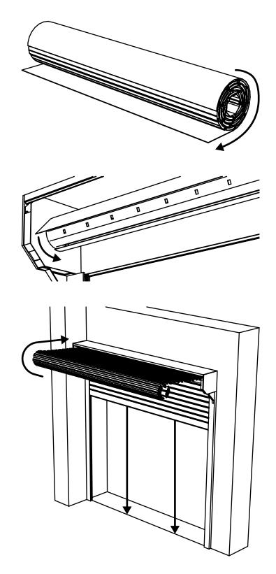
D. Remove the soft protective material you wrapped around the axle (E) in step B on the previous page.
