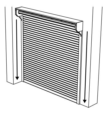
J. Install the auto-lock brackets (L) onto each side of the box housing (A). Ensure the shutter is in the closed position.
