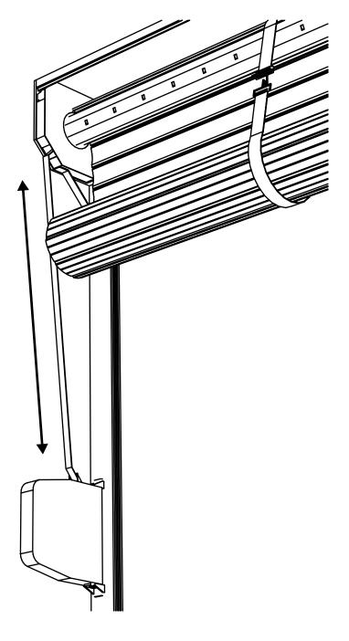
G. Using the tape, carefully rotate the axle(E). This will transfer the curtain roll (B)from the straps onto the axle.
