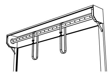
B. Lift the curtain roll (B) up and into the strap loops. The curtain roll should be orientated so that the loose end of the curtain is coming up the back of the roll. Let the straps take the weight of the curtain roll so that it is hanging from the axle (E). Ensure the straps are in no danger of slipping.
