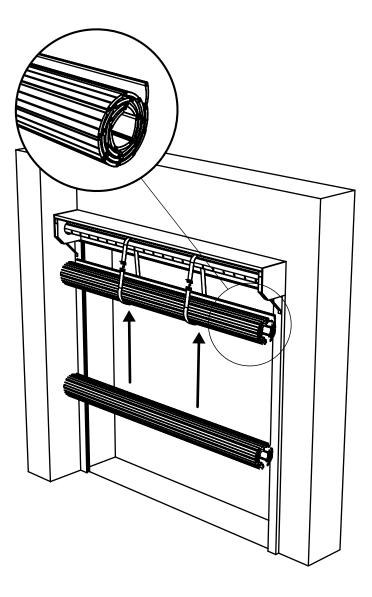
C. Slide the t-clips (H) provided onto the top of the curtain. Evenly space them along the width of the curtain with the end ones 3" in from each end of the curtain.
