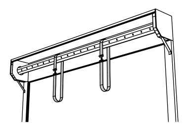
C. Lift the curtain roll (B) up and into the strap loops. The curtain roll should be orientated so that the loose end of the curtain is coming up the back of the roll. Let the straps take the weight of the curtain roll so that it is hanging from the axle (E). Ensure the straps are in no danger of slipping.
