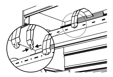
H. Using the charging handles, carefully rotate the axle (E) the opposite way, until you feel the spring tension transfer onto the curtain. Remove the charging handles and allow the curtain to coil up into the box housing (A).
