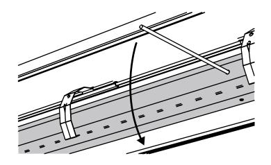
I. Install the auto-lock brackets (L) onto each side of the box housing (A). Ensure the shutter is in the closed position.
