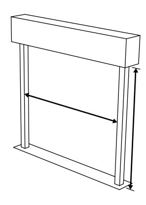
You will need the depth of one guide rail on each 3x3 post, and the curtain will coil up in the ceiling/bulkhead onto an EntrexGuard axle. The shutter is installed between the 3x3 posts.
