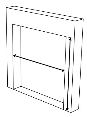
You will need the depth of one guide rail on each side of the opening, and the depth of the box housing at the top of the opening.
