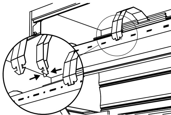
6. Using the charging handles, carefully rotate the axle (E) the opposite way, until you feel the spring tension transfer onto the curtain. Remove the charging handles and allow the curtain to coil up into the box housing (A).
