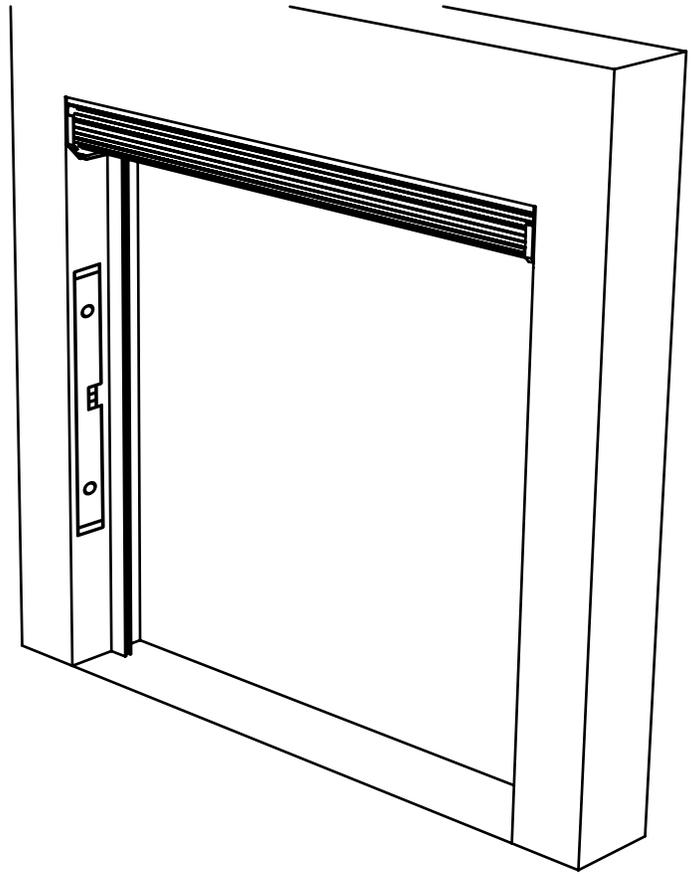
7. Mount the guide rails (C) to the sides of the opening. Use the #10 - 2" screws (J1) provided to secure the guide rails to the opening.
