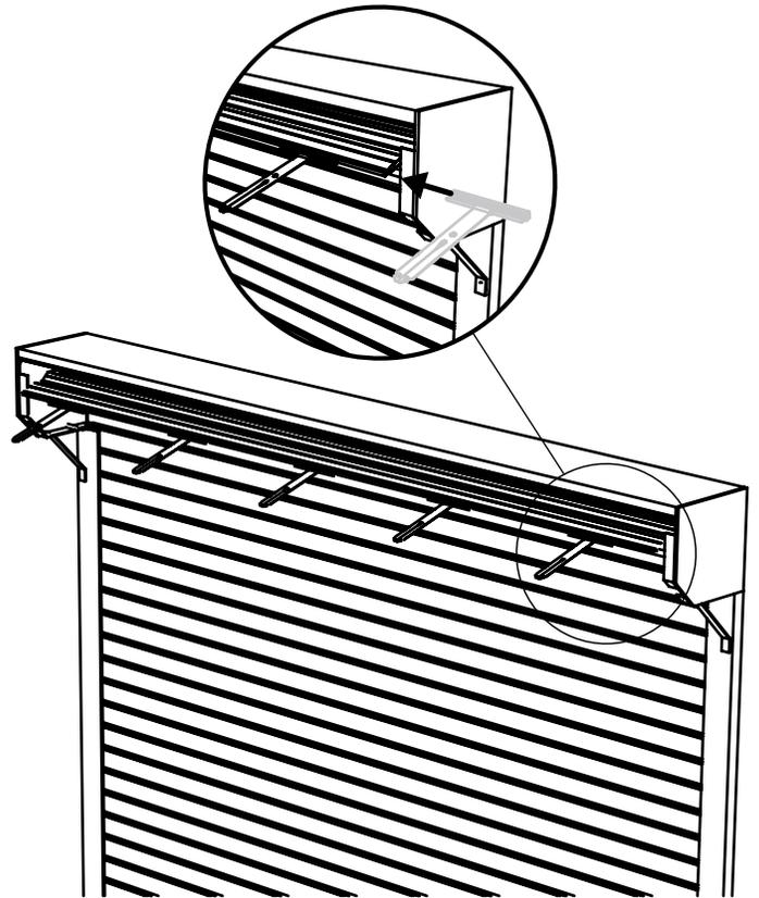
8. Before attaching the curtain to the axle (E) you must tension the axle spring by turning it with the charging handles provided.
