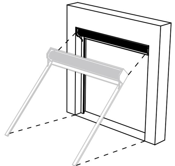
6. Ensure the box housing (A) and guide rails (C) are straight and level. Use shims if required to keep the guide rails straight.
