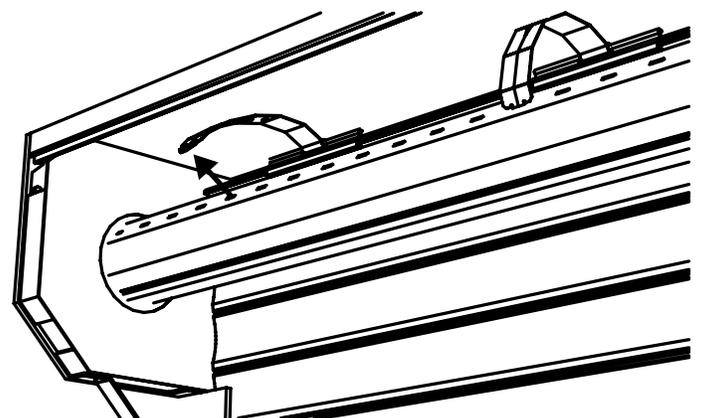
4. Insert the charging handles into the axle (E) again, and turn the axle the opposite way by moving the handles down from the top of the box housing (A) to the curtain. Continue turning the axle for one complete turn (360 degrees).
