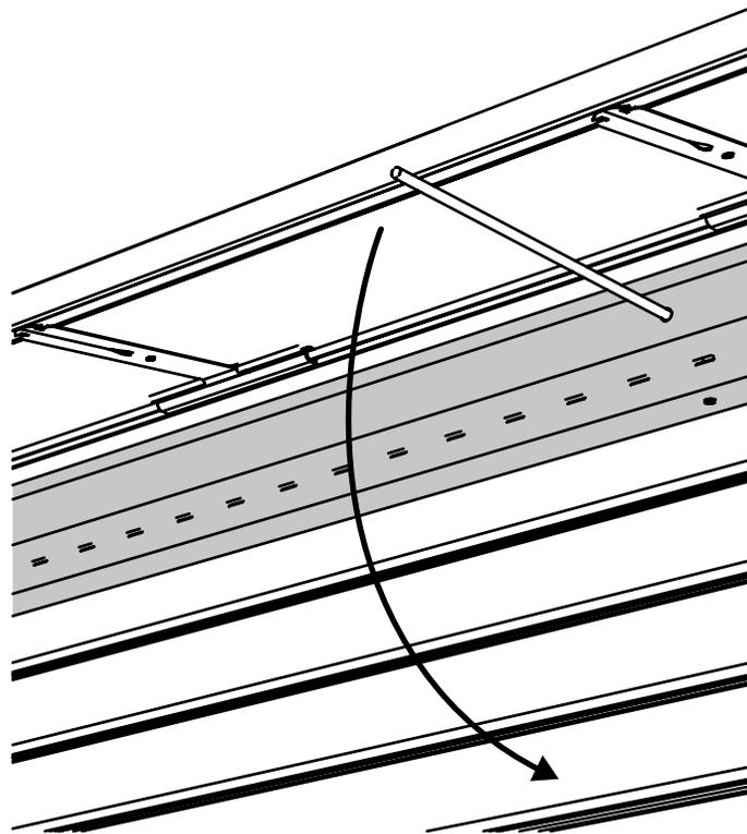
5. Reattach the t-clips (H) onto the axle (E) by squeezing the arrow-shaped ends, and inserting them into the long narrow slots in the axle.
