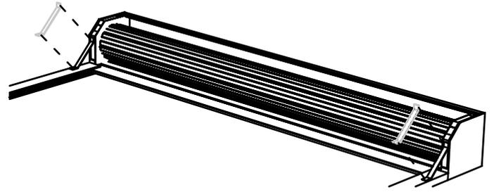
5. Lift the shutter up and into position over the opening by holding the box housing (A) and guide rails (C) and slowly rotating the entire shutter 90 degrees, so it is standing up vertically.
