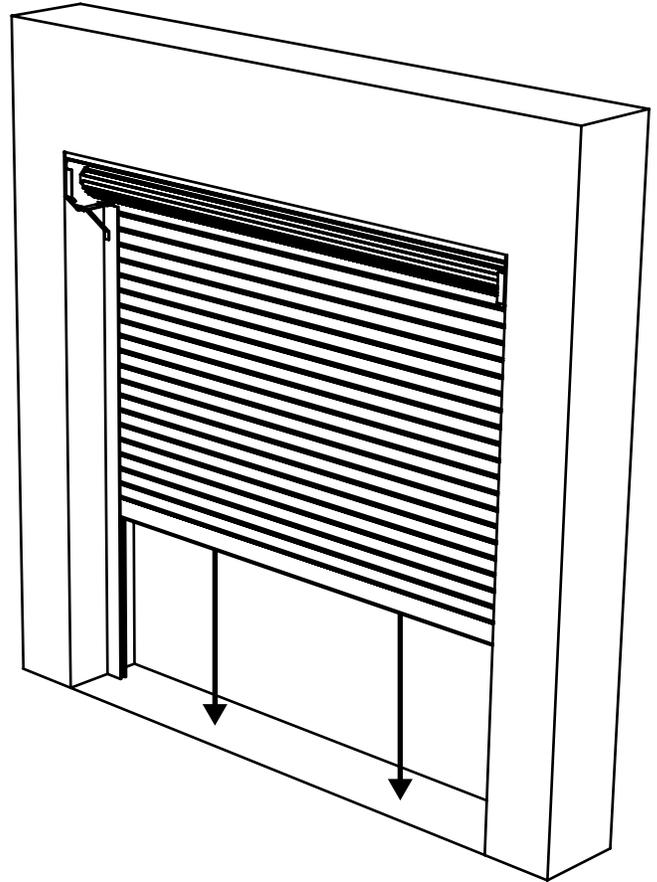
10. Mount the box housing (A) to solid backing with a screw at each end, and one screw every 16" across the width. Use the #10 - 2" screws (J1). Insert the screws through the top of the box housing.
