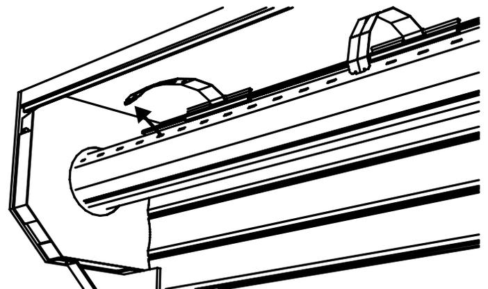
4. Insert the charging handles into the axle (E) again, and continue turning the axle by moving the handles up from the curtain to the top of the box housing (A). Turn the axle for one complete turn (360 degrees).
