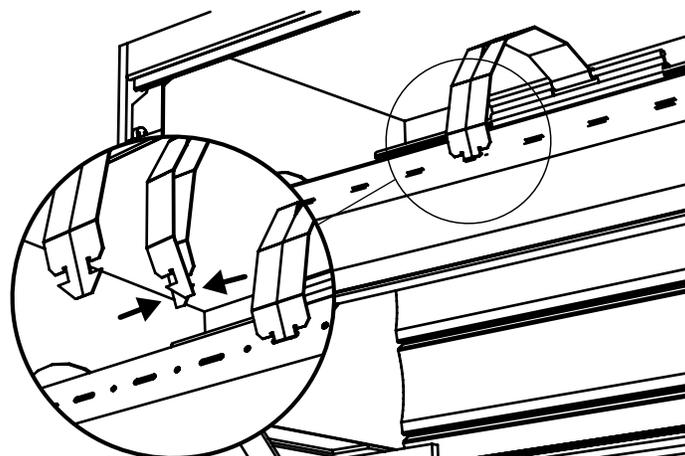
10. Using the charging handles, carefully rotate the axle (E) the opposite way, until you feel the spring tension transfer onto the curtain. Remove the charging handles and allow the curtain to coil up into the box housing (A).
