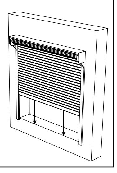
10. Mount the box housing (A) to solid backing with a screw at each end, and one screw every 16" across the width. Use the #10 - 2" screws (J1). Insert the screws through the back of the box housing.
