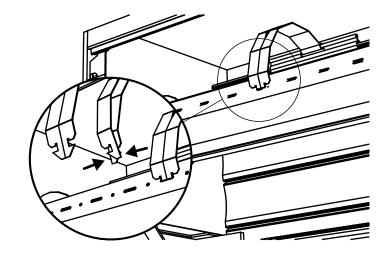
G. Using the crank handle, carefully rotate the axle (E). This will transfer the curtain roll (B) from the straps onto the axle.
