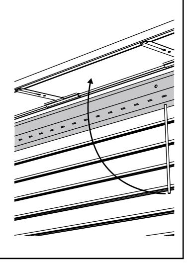
G. Attach the t-clips (H) onto the axle (E) by squeezing the arrow-shaped ends, and inserting them into the long narrow slots in the axle.
