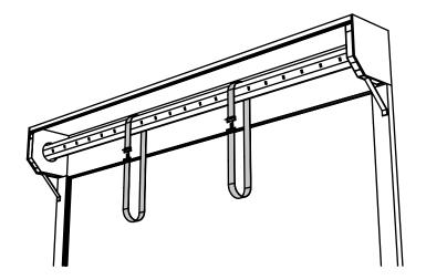
C. Lift the curtain roll (B) up and into the strap loops. The curtain roll should be orientated so that the loose end of the curtain is coming up the back of the roll. Let the straps take the weight of the curtain roll so that it is hanging from the axle (E). Ensure the straps are in no danger of slipping.
