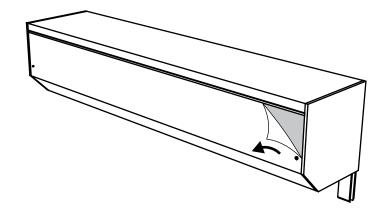
2. Ensure the entire mounting surface is completely flat. You will need the width of one guide rail (C) on each side of the opening face, and the height of the box housing (A) above the opening.
