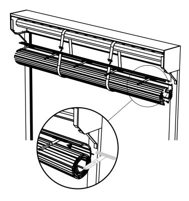
E. Rotate the curtain roll (B) in the straps and pull the loose end of the curtain roll up behind the axle (E).
