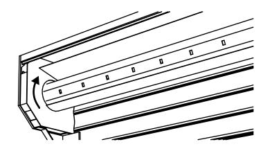
E. Slide the t-clips (H) provided onto the top of the curtain. Evenly space them along the width of the curtain with the end ones 3" in from each end of the curtain.
