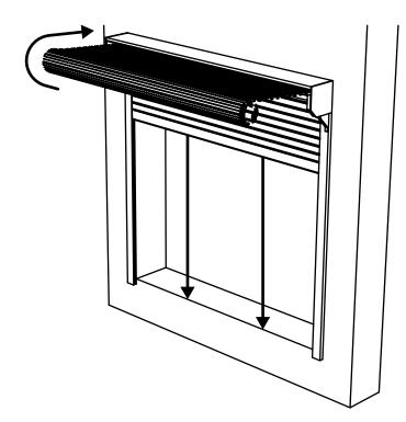
D. Remove the soft protective material you wrapped around the axle (E) in step B on the previous page.
